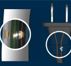
Series Arc: Arc along the same conductor or at connections
