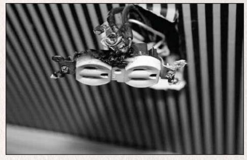
and mid-1970's to include aluminum wiring. If you are unsure whether your home is among them, look at the printed or embossed markings on the outer jacket of the electric cables, which are visible in unfinished basements, attics, or garages. Cable with aluminum conductors will be marked on the sheath with "Al" or "Aluminum" along its length. If you are unable to determine the type of wiring, contact a qualified electrician to investigate.
